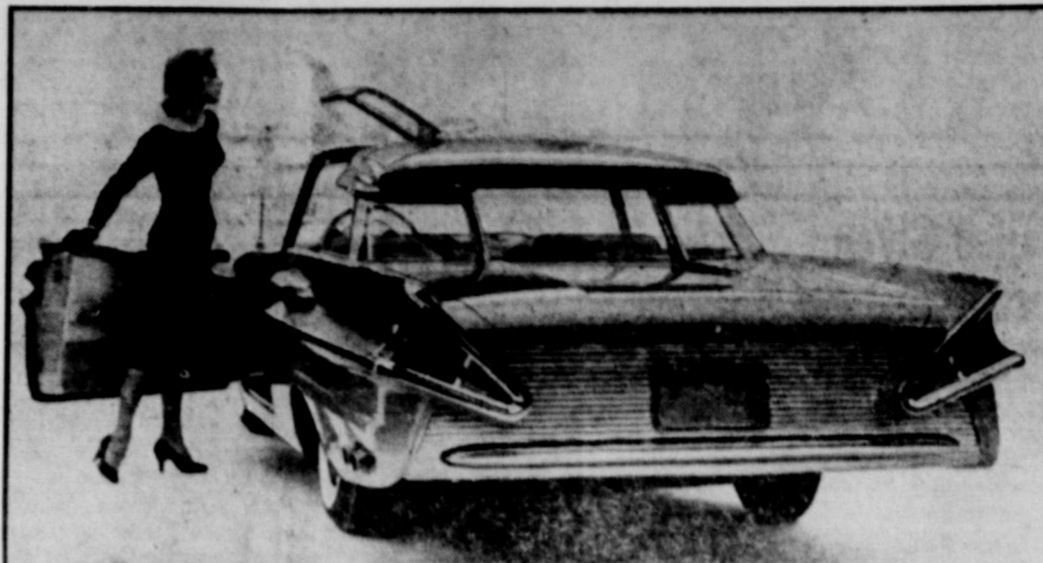
GEARED TO TOMORROW —Scoop-channel sidewalls and fenders, "butterfly" roof inserts which rise as doors are opened and turn-and-stop lights at left and right-hand corners of roof mark the striking design of Mercury's experimental XM-Turnpike Cruiser. Only 44 feet high, the car is styled to meet roll across the nation's ever-expanding highway system. Other features: Side-vent exhaust beside left-rear wheel and windows which wrap around corners usually occupied by frame posts. First shown in Chicago, the machine will be put on a nationwide display tour.
