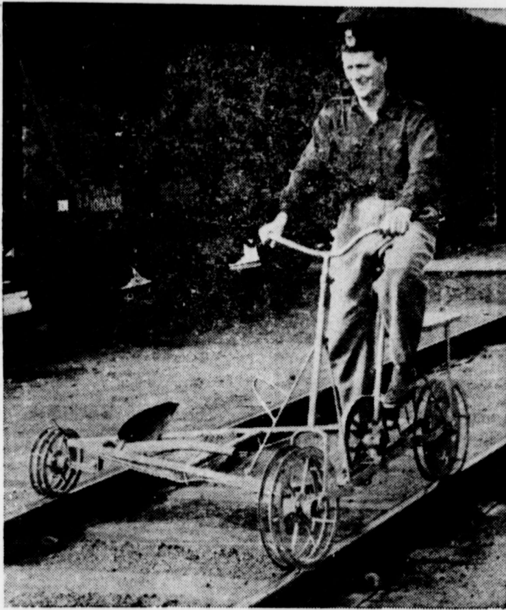
MAKING TRACKS —Railroad worker Birger Sandman rides to the job on a special tricycle in Kiruna, Sweden. The town, 90 miles north of the Arctic Circle, depends completely on the railroad to bring in supplies.
