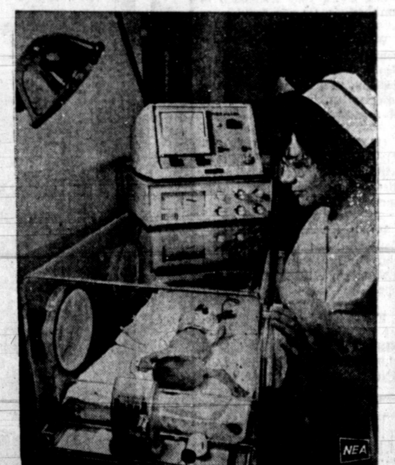
NEW CHANCE is given premature infants suffering from respiratory disorder, by monitoring their breathing with a new electronic device. Developed by a Stanford University research team in Palo Alto, Calif., in co-operation with two San Francisco Bay Area electronic firms, it is designed to keep close watch on performance of tiny youngsters, such as this one at Palo Alto-Stanford Hospital Center, to prevent death or brain damage.
