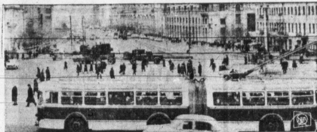
RED, RED, RED IS THE TROLLEY—When they're not riding in Moscow's sumptuous subways, Muscovites do their commuting in trolley buses, first introduced some 30 years ago. A new wrinkle is the tandem trolley with an accordion bellows coupling. This bus can carry 180 passengers.
