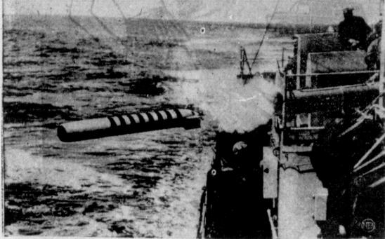
GOING "HOME"-A new lightweight acoustic-homing torpedo, developed by the U.S. Navy, leaves the firing tube aboard the USS Tweedy and begins its unerring journey to its target. The development of the new surface-launched torpedo is part of Navy's program of continually improving its anti-submarine weapons. The new weapon is already in use by the fleet. In releasing this photo, the Navy did not locate the scene of the action.
