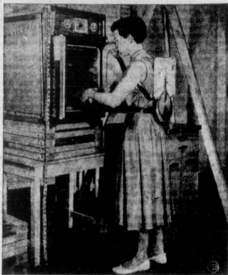
Every breath she takes is measured by portable respirometer as Department of Agriculture household equipment specialist evaluates adjustable oven installation in test kitchen at Washington, D.C. Tests indicate that ovens 28-40 inches from floor are least fatiguing for homemaker to use.
