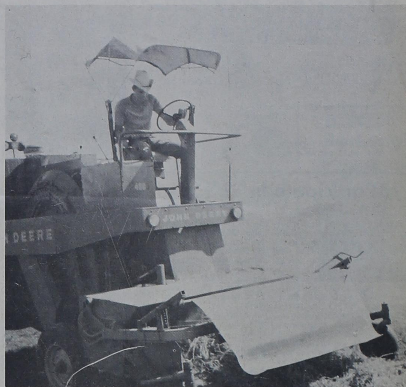
HAY CUBING -- Albert Lee, one of the five men employed by the Prince-Abbott firm in its hay cubing operation, works at the Loyd Stevens farm south of Farwell operating the cubing machine. The machine, in one process, picks up and manufactures the freshly cut alfalfa into cubes. The firm has two machines in operation in the area south of Farwell, where most of the cubing has been done this year. The operation began in May and is expected to continue through September.
