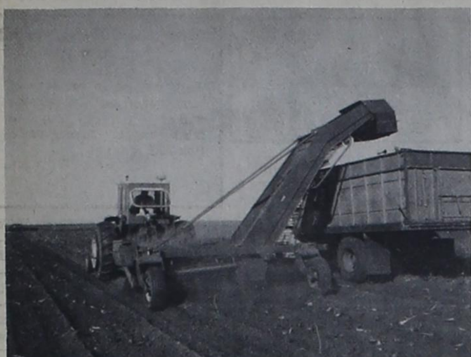
DIGGING BEETS -- A tractor-pulled machine conveys sugar beets from ground to truck to be hauled to the nearest railway point for transportation to the sugar beet processing plant in Hereford. Sugar beet harvest in the area has been in full swing with many loaded railroad cars seen on the sidings every day. Sugar content in the beets has not reached the desired levels yet, but it is some improved over last year's crop.
