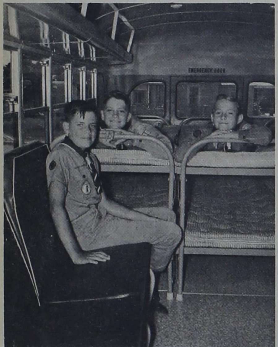
READY FOR ANYTHING -- Texico-Farwell Troop 200 changed a "school" bus into a Scout bus by installing a continuous vinyl floor over foam padding, providing six bunk beds for travel comfort and unexpected conditions, adding new paint inside and out, and completely rearranging seats to face inward and thereby provide extra floor space. Scouts (l to r) Donnie Garner, Randy Stovall, and David Turnbough take a well-deserved rest in the bus, after helping sell 2,592 boxes of candy toward its purchase.
