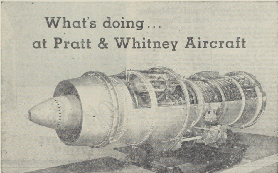
Cutaway model of P & W A J-57 engine. This twin-spool, axial-flow gas turbine powers the country's newest fighters and bombers and is slated for Douglas DC-8 and Boeing 707 jet airliners. Engine was the first to be rated at more than 10,000 pounds thrust.
