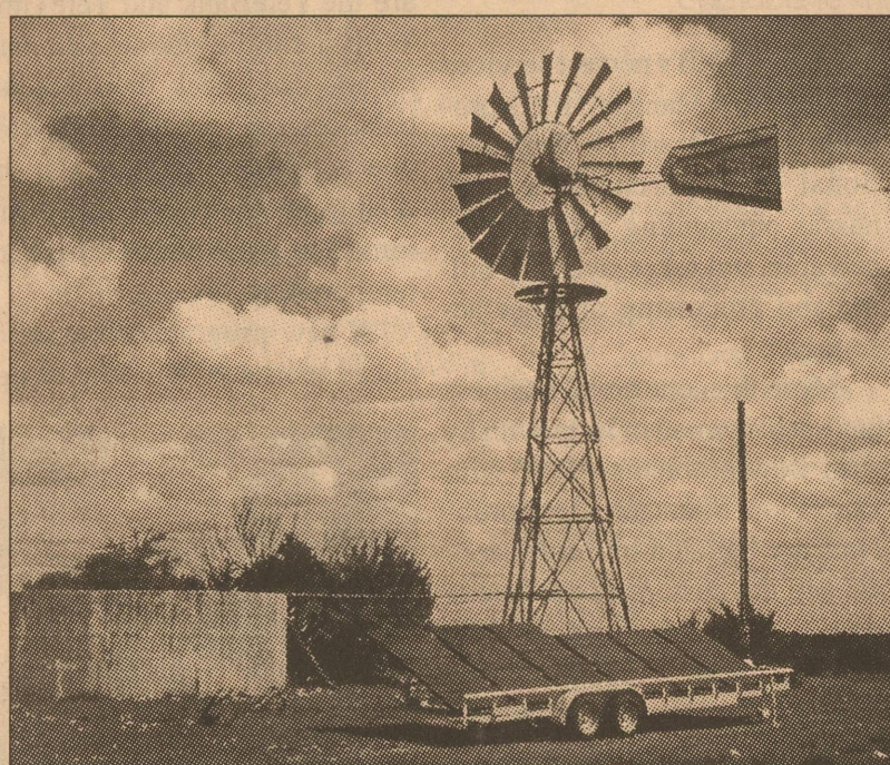
Southwest Texas Electric Cooperative has these photovoltaic panels mounted on a trailer to test with any submersible pump. Call today for a demonstration.
