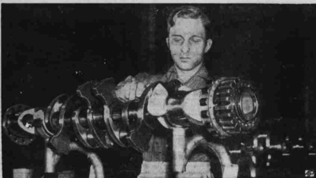
PART OF PLANE'S POWER —Close-up shows build of crankshaft that takes the pounding of 12 cylinders in Allison plane engines being turned out at rate of 350 a month in Indianapolis.
