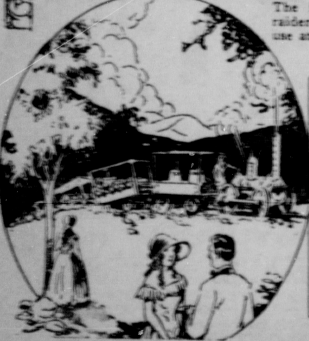
The first engine ever run in America—the "Tom Thumb," built by Peter Cooper in 1830, which could pull 40 people 15 miles an hour over the Baltimore and Ohio.
