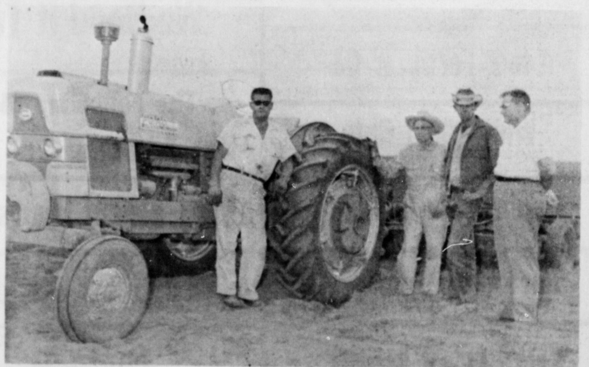
A demonstration on the Rufus Carter farm 3 1/2 miles east of Lubbock showed the Ford 6000 would pull a 14 foot tandem at 5.2 miles per hour. Left to right are Bennie St. Cyr, field supervisor, Mr. Carter, owner of the farm, Jr. Davis, who has the farm leased, and Hollie Francis, owner of Francis Implement Company in Muleshoe.
