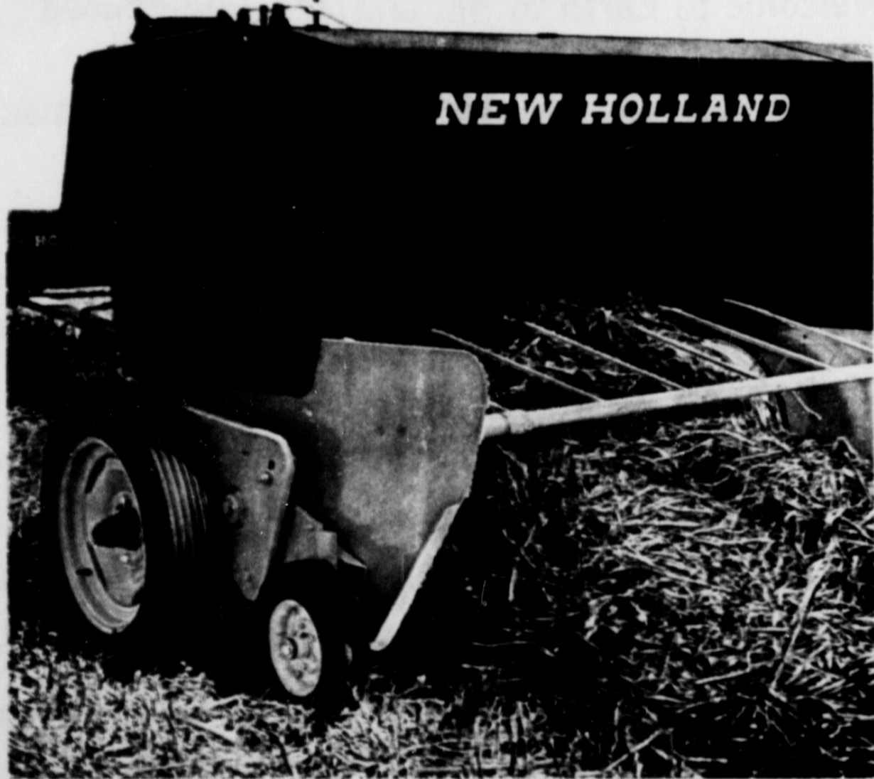
Hayliner 271-14" x 18", twine or wire, engine or P.T.O.; bale-thrasher optional.
