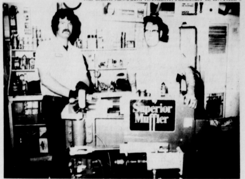
Possibly the newest innovation in the muffler and tailpipe business has been installed at Earth 66. Owners Harold and Brian Britton are shown here as they make ready to form a new tail pipe. The machine is capable of bending from pattern or computer card as well as custom bending to almost any form. Harold Britton, who has been in business in Earth for the past thirteen years, is justifiably proud of this new equipment and welcomes everyone to come by and he will be happy to explain its operation.
