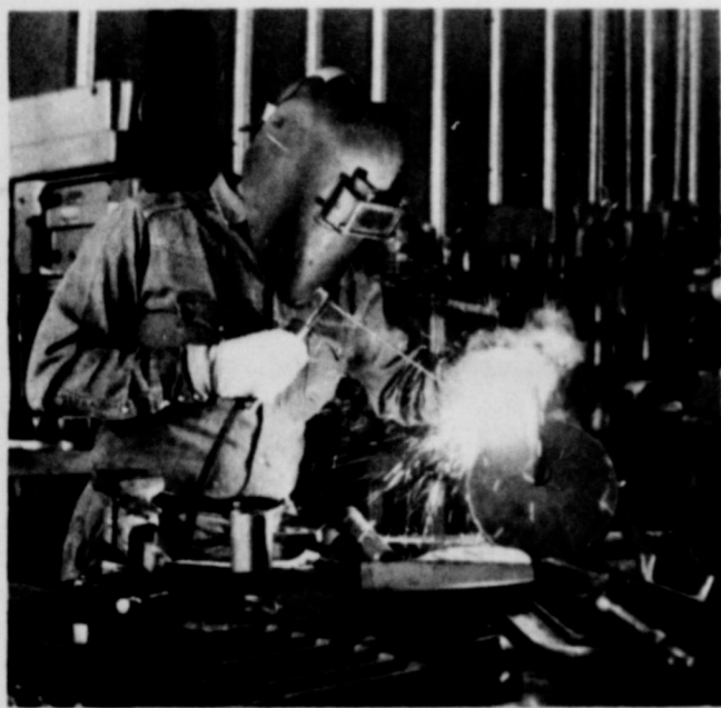
DEE LOTT, Shop Foreman, welding secondary end plates, prior to a machinery operation.
