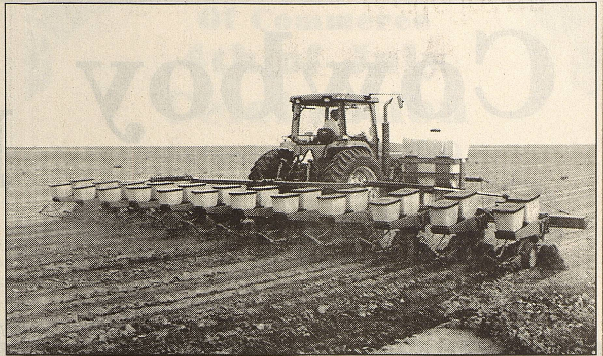
This John Deere tractor and twelve row planter were busy Monday morning just east and north of Tokio planting sunflowers on hailed out cotton acreage
