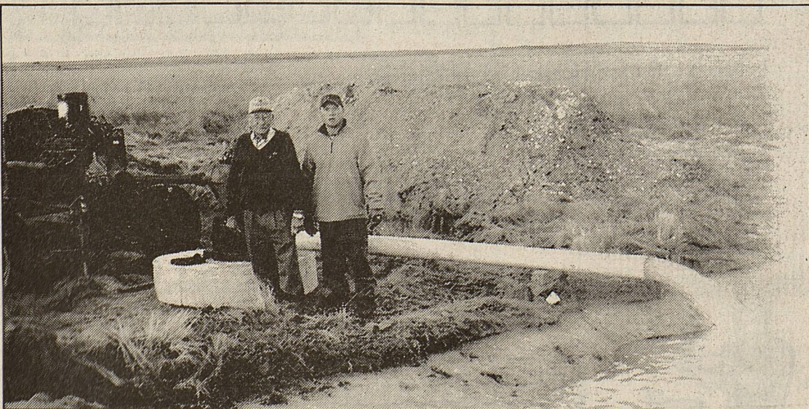
Land owner Bob Blundell, left and tenant-producer Sterling Lovelace are seen running tests on recently drilled irrigation well in northwest area of county. The well was producing about 700 gallons per minute during the test.
