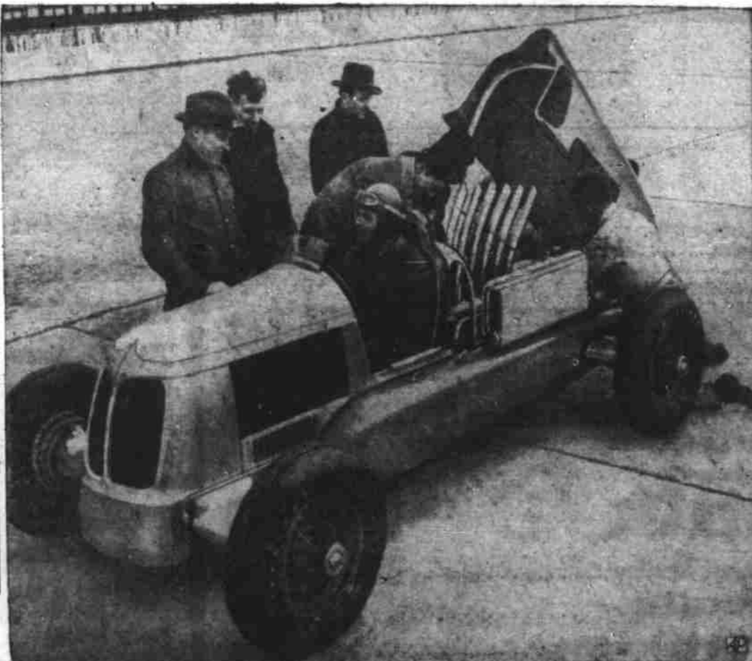
WITH ITS MOTOR AT THE REAR , one of the three rear-motor racers to be entered by Harry Miller in the Indianapolis Speedway May 30 gets a going-over by George Campbell (at wheel). The car is of four-wheel drive construction, and six exhaust pipes streamline out of the hood in back of driver. Pontoon-like gas tanks line left and right sides of chassis.
