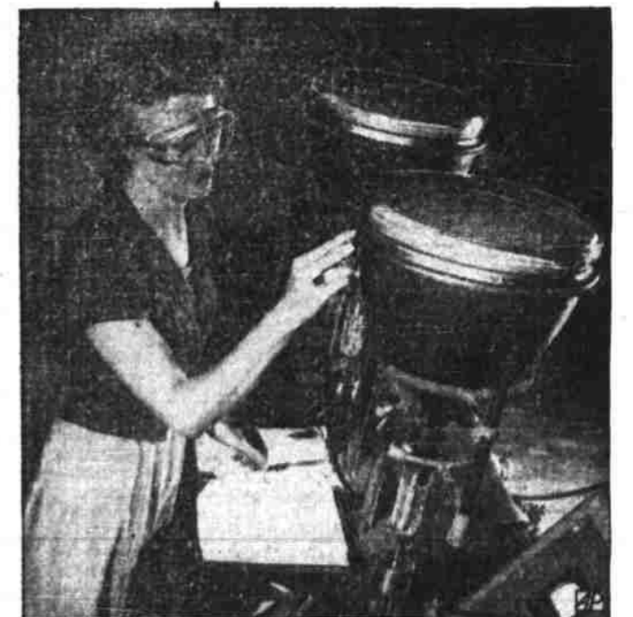
AIRTIGHT CHECK — A worker at RCA Lancaster, Pa., plant checks a tri-color TV picture tube under vacuum to make sure of airtight weld between main cone and screen section.
