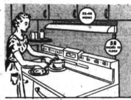
AT THE RANGE: A shielded light unit placed as shown over the range makes a lighting recipe that helps cooking recipes! The whole range top is illuminated—you can see into pots and pans.
