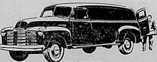
MEDIUM-DUTY PANEL Model 3805—137-inch wheelbase, Maximum G.V.W. 6700 lb. Also available in light-duty Model 3105—116-inch wheelbase, Maximum G.V.W. 4600 lb.
