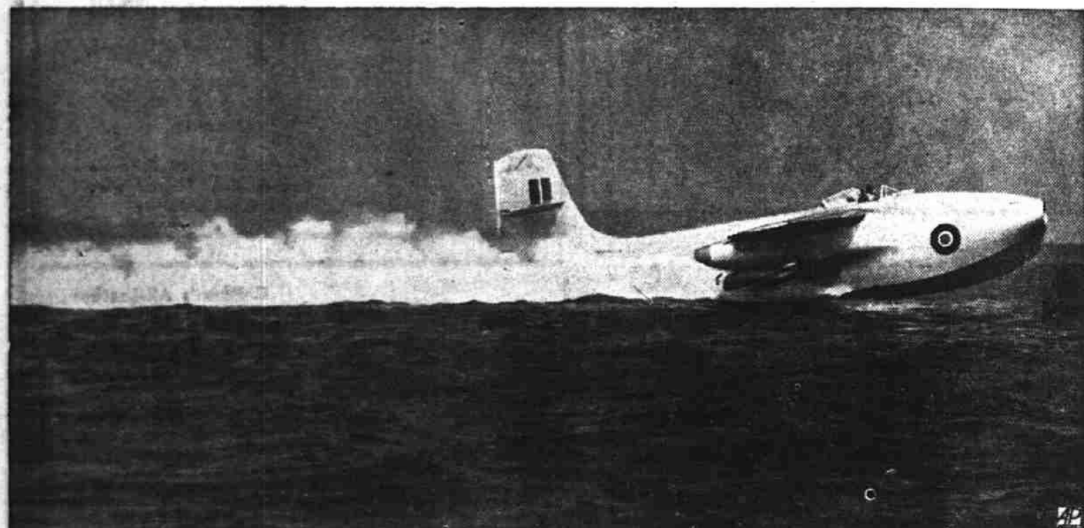
BRITISH JET FLYING BOAT — The Saunders-Roe A1, Britain's jet flying boat fighter, undergoes a successful test off the Isle of Wight. The boat has two jet units and four 20-mm. cannon fitted in the nose.
