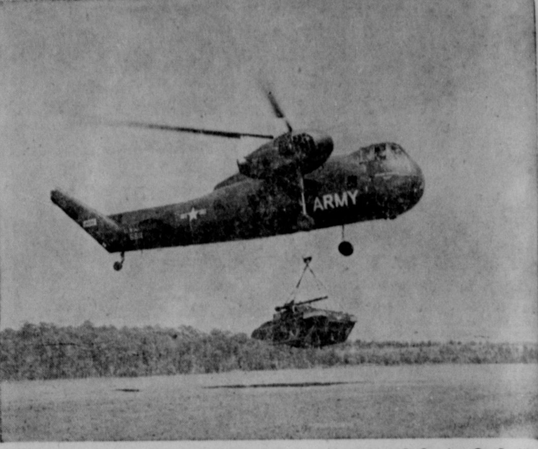
New way to move tanks over short distances is developed by Army at Ft. Benning, Ga. Participants: H-37 helicopter and M-56 tank. Latter totes a 106-mm recoilless rifle.
