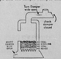
be open wide. If the ashpit damper on your furnace is in back, open it and also the ashpit door in front. This assures maximum draft and quick ignition.
