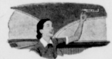
Grilles in Buick's exclusive dual roof ducts insure draft-free distribution of conditioned air—and also provide individual control of air direction as desired.
