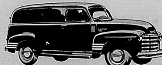
LIGHT-DUTY DE LUXE PANEL* Model 3105—116-inch wheelbase, Maximum G.V.W. 4,600 lb. Also available in Medium-Duty model 3805—137-inch wheelbase, Maximum G.V.W. 6,700 lb.
