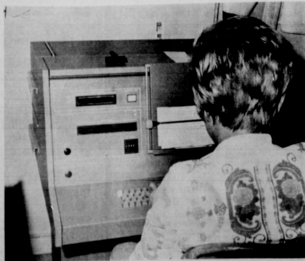
NEW TYPESETTING EQUIPMENT --- The Slatonite this week began using a new Compuwriter, an electronic photo-typesetting machine which will replace the machines used for the last eight years to set type. Readers should notice the difference in the small type like this. The new equipment makes it possible to set the type for the newspaper faster, neater and cleaner. Lenda Wood is operating the machine here. (SLATONITE PHOTO)
