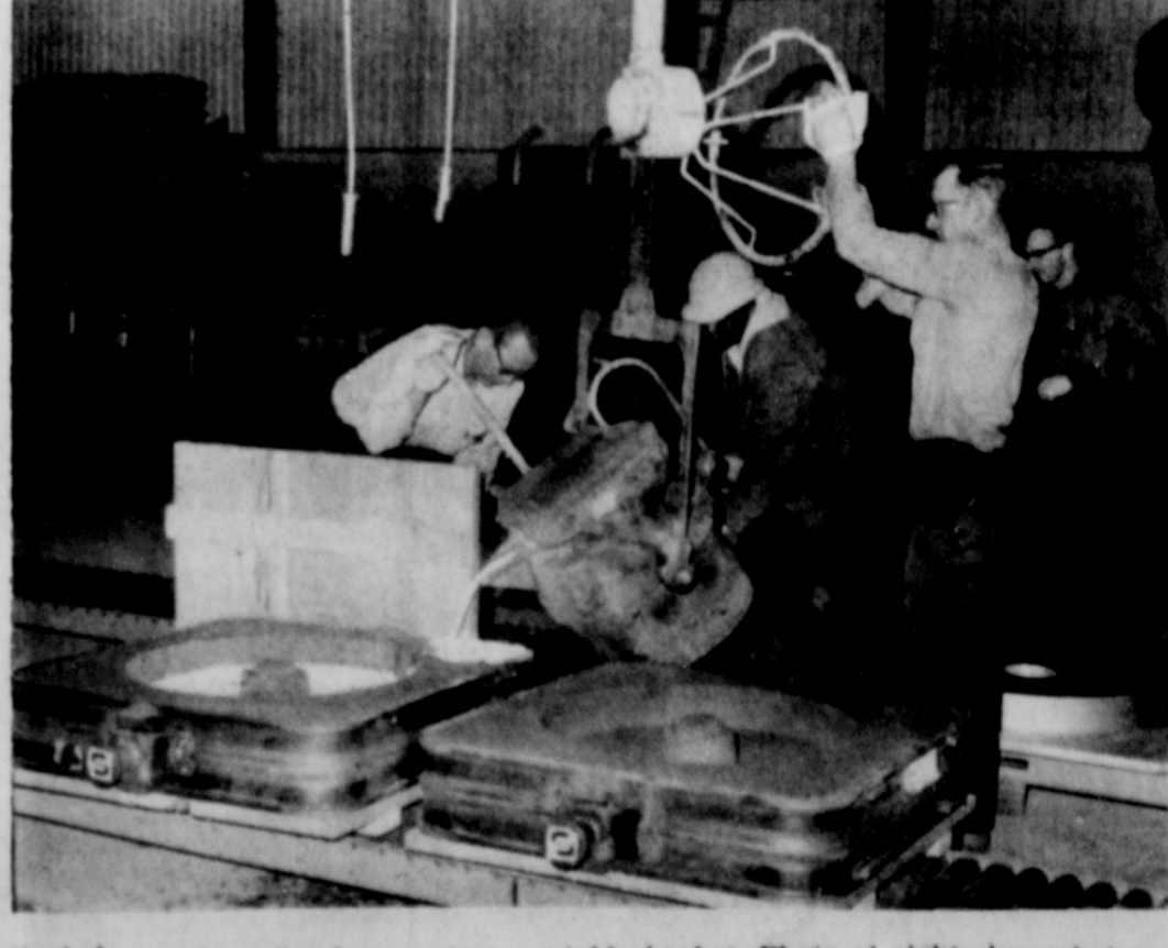
from the furnace to a portable bucket. Photo at right shows hot metal going from bucket into the mold, which is formed from a special mixture of sand. (Slatonite Photos)
