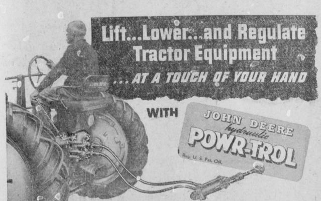
Think of it! A touch of your hand raises and lowers such equipment as plow bottoms, cultivator shovels, mower cutter bars, combine platforms, and corn picker ge herers ... angles and straightens disk harrow gangs ... instantly changes working angle, depth or height to meet varying field and crop conditions!
