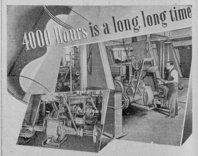
FOUR thousand hours is a long time to keep a tractor operating at high speed, at peak load. But, that is the break-down test new models of John Deere Tractors must pass before they are ready for production-4,000 hours without failure.
