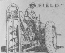
attach on any farm tractor with rear-end power take off. Digs holes in hard dry soil. It's easy to set the depth gauge and control all operations from the driver's seat. Interchangeable auger sizes . . . Timken bearings.
