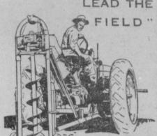
They are easy to attach on any farm tractor with rear-end power take-off. Digs holes in hard dry soil. It's easy, to set the depth gauge and control all operations from the driver's seat. Interchangeable auger sizes . . . Timken bearings,
