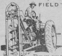
attach on any farm tractor with rear-end power take off. Digs holes in hard dry soil. It's easy, to set the depth gauge and control all operations from the driver's seat. Interchangeable auger sizes . . . Timken bearings.
