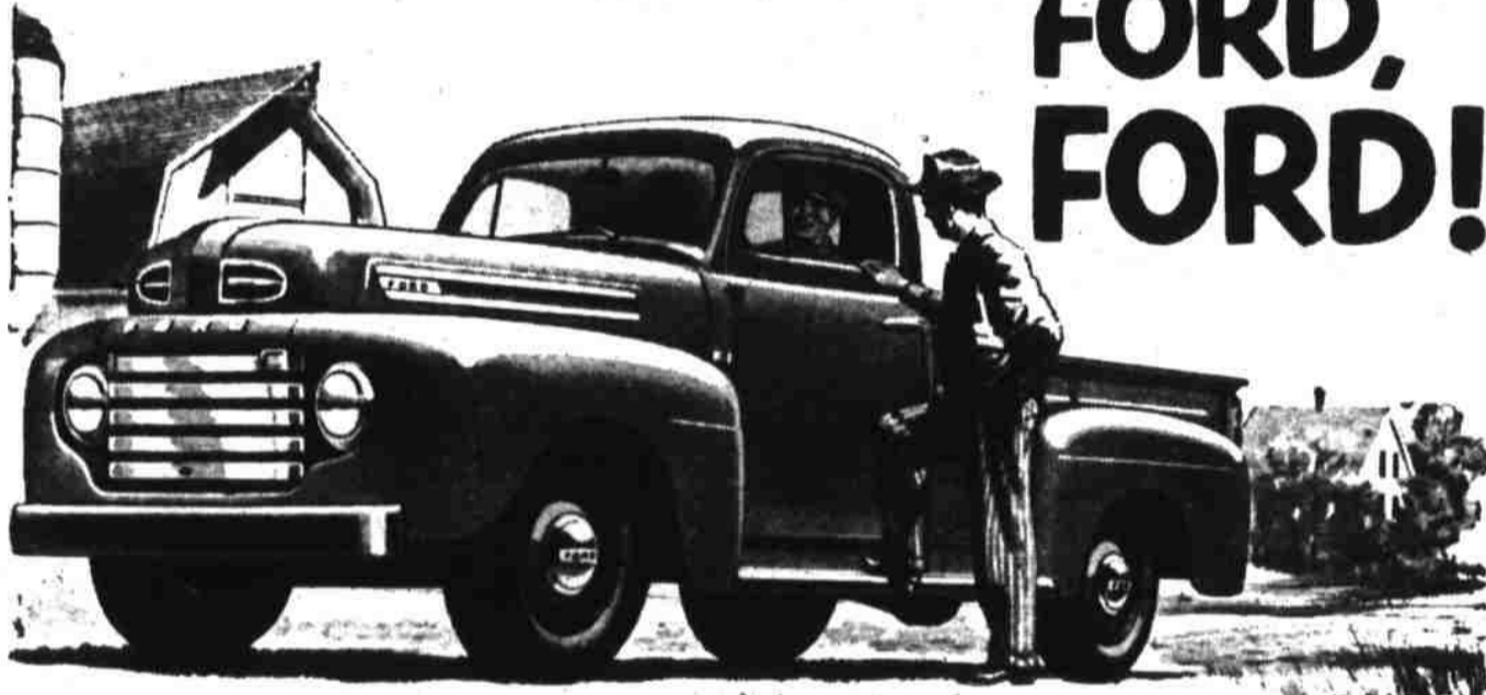
6 1/2-ft. Ford F-1 Pickup shown here. G.V.W. rating—4,700 lbs. Body capacity—45 cu. ft. Available with 95-h.p. Six or 100-h.p. V-8. One of over 175 models including 145-h.p. Big Job.
