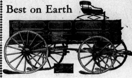
Made of good seasoned timber. Metal covered hubs, which will not crack or check, two-piece fellow, patent outer bearing axles, oak hubs, spokes and fellows. Hubs are cupped behind, forming sand protection. Spokes closely fitted and dirven in hot glue. Rivets on each side of spokes. Hub band put on hot. Seamless cast skein. Every wagon we sell has a full guarantee. Come, let us show you all the good points about these wagons.
