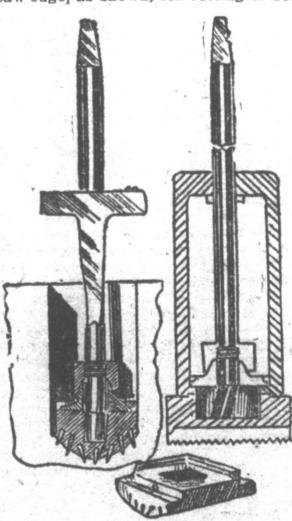
ing into the wood, and the others have a smooth edge for clearing away the fragments. As the spindle rotates, a rocking motion is imparted to the head, so that a rectangular hole may be formed in the wood.
