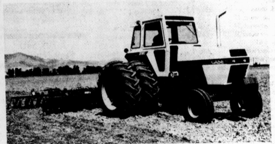
The Case 2090 with 108 PTO Horsepower
