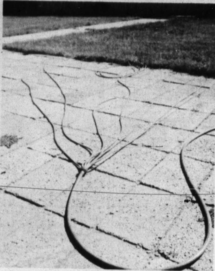
OCTOPUS WATERER - This pale green waterer feeds shrubs such as roses with long smaller tubes, giving it the name of octopus. The 'feelers' are virtually invisible among the plants and supply a slow stream of water. See story this page. (Staff Photo)
