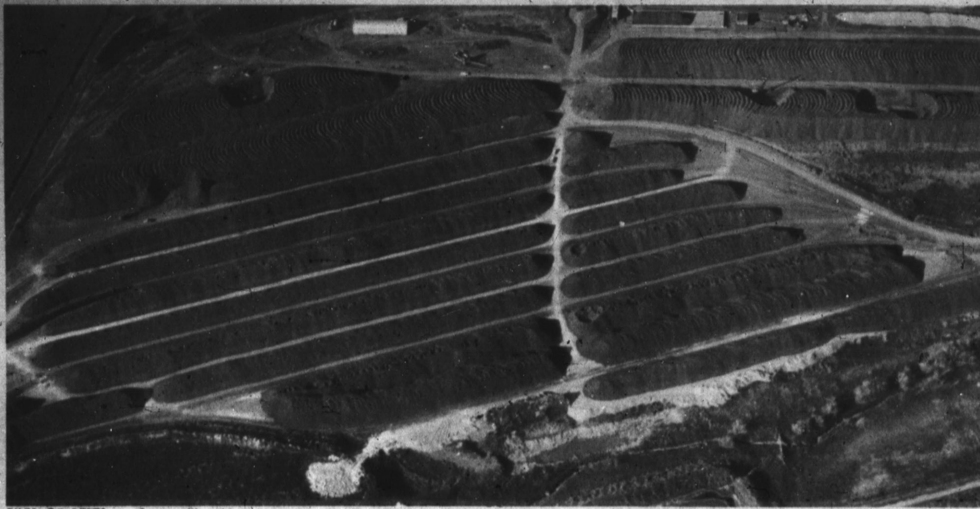
FILES OF BEETS.— Scenes like this will appear at the Mettrill E. Shoup Plant of Holly Sugar Corporation in a few weeks as the sugar beets begin to arrive at the newly constructed factory. The beets are stored in huge outdoor piles during the harvest season and then moved into the factory for processing as needed. This view shows the beets that are stacked 20 feet high. From the piles, beets are flumed into plant in water which starts the cleaning process even as it transports the roots to the refinery. (Holly Corporation Photo)
