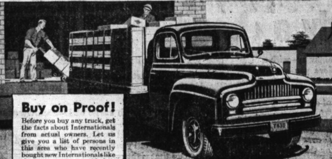
Model L-162, 154-in. wheelbase, 12-ft. stake body, 16,000 lbs. GVW.
