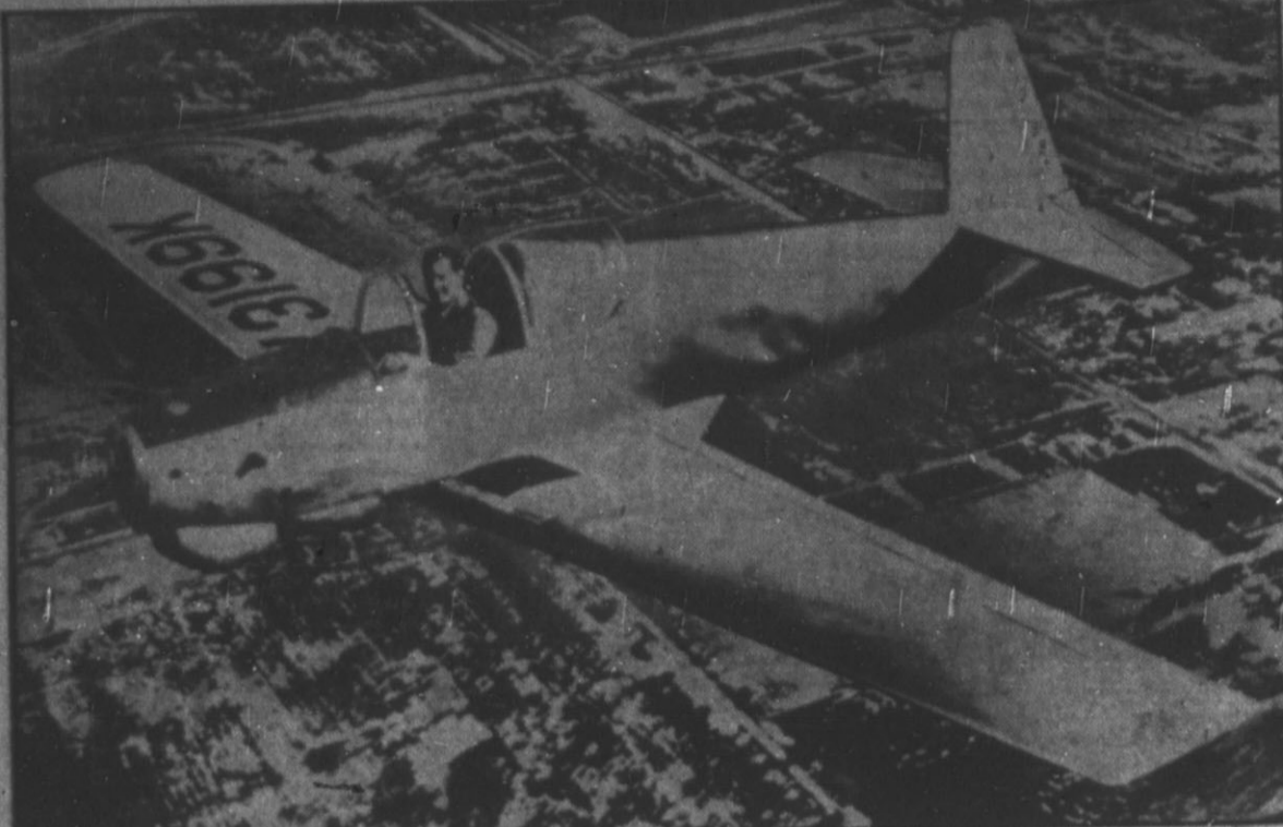
Test pilot Bill Taylor puts this tiny M-18, powered by an automobile engine, through its paces 2000 feet over Wichita, Kan. The rugged little one-seater flier has a 27-foot wingspan, weighs only 450 pounds, and has a retractable landing gear and single-lever control. It can average 100 miles an hour, yet the designer claims it will cross the country on $12 worth of gasoline.
