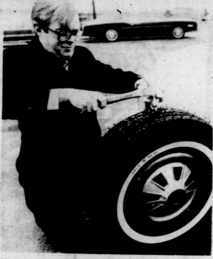
WHY IS TOM REESE pounding nails into one of the tires manufactured by his company? To prove his contention that the tire is nearly indestructible. According to Reese, as many as half of the new cars sold by 1985 could be equipped with similar self-sealing tires that prevent air loss in most tread-area punctures.
