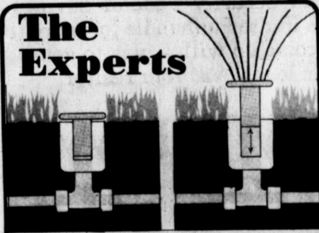
UNDERGROUND SPRINKLER SYSTEM
