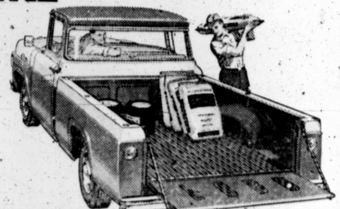
'59 Ford Style Side is roomy—and rugged! Wrap-around rear corners with rigid box-girder-type construction strengthen both body and tailgate.
