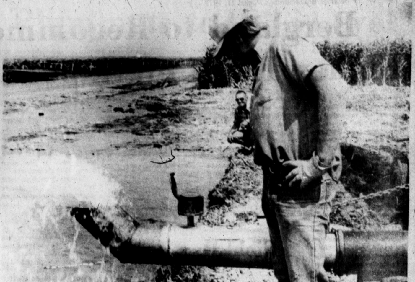
Don Oppliger, foreman at the Gerk farm, takes a reading on the well's pumping capacity as water gushes from a metered extension on the discharge pipe. Water meters are an import tool in measuring the productivity of newly developed
