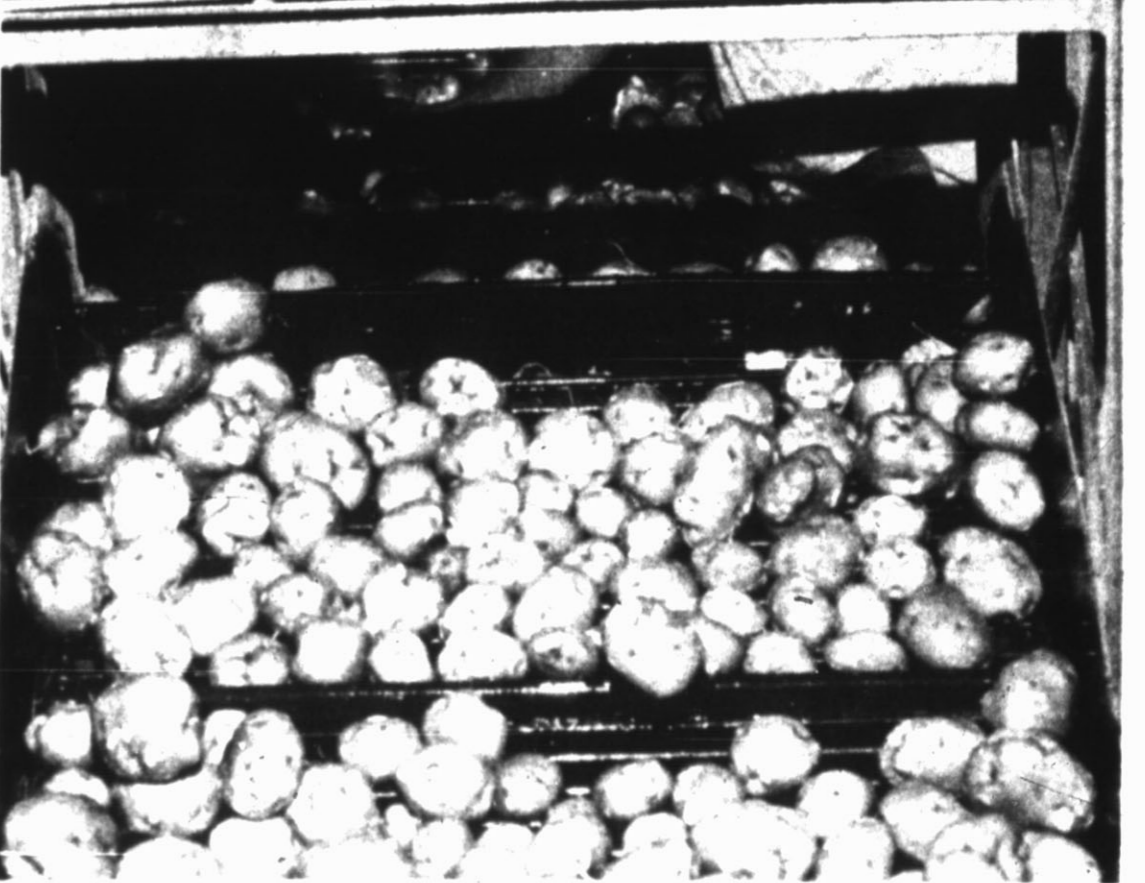
LARGE HEREFORD POTATOES come streaming through the processing line after getting a good scrubbing. From this point they are sorted both manually and mechanically, then bagged in 50 or 100-pound sacks for shipment by truck and rail all over the United States.
