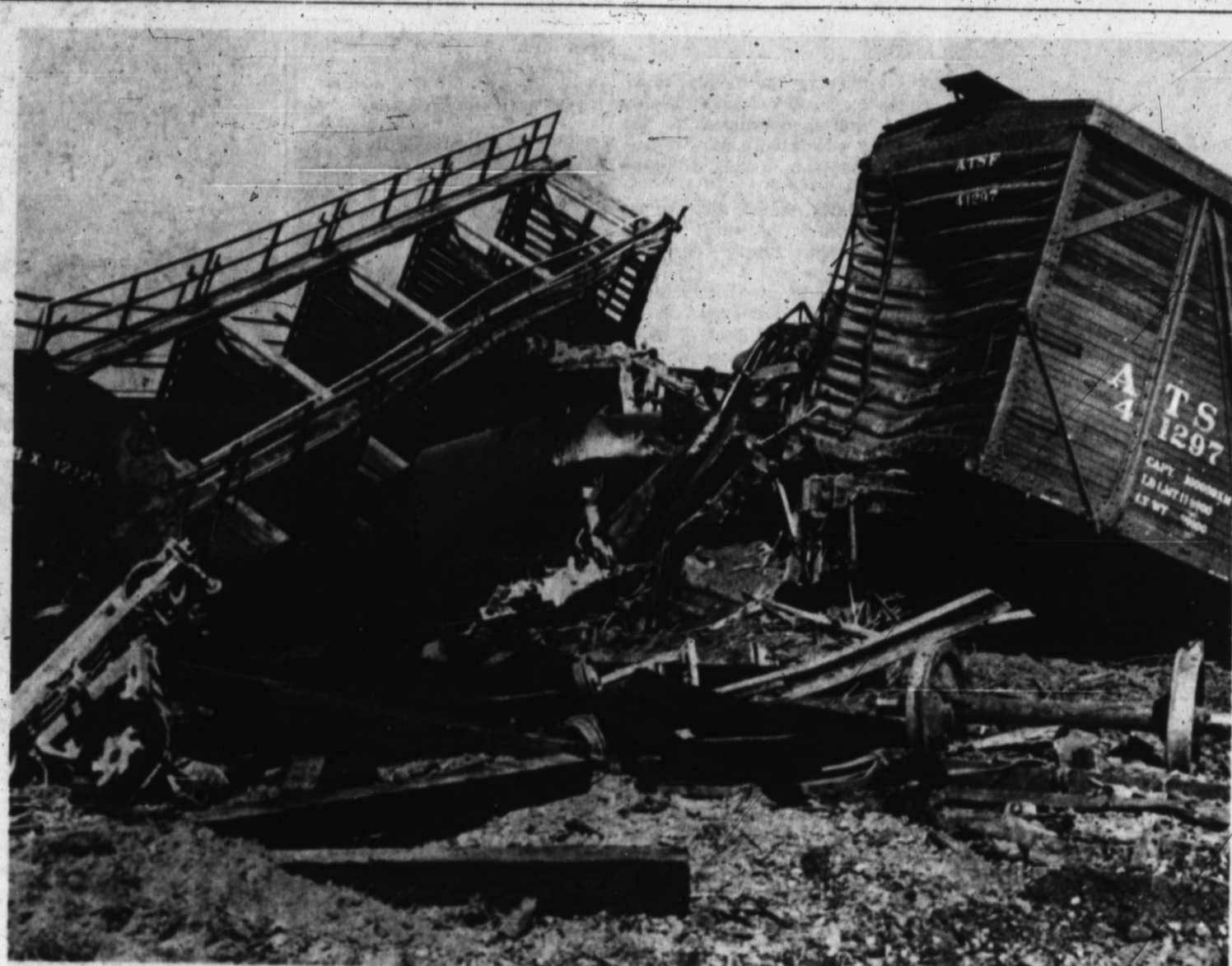
A 40-CAR TWISTED wreckage was all that remained of 40 cars after a derailment caused apparently by a faulty journal on one of the cars. The accident occurred about seven miles southwest of Hereford as a speeding 128-car freight was approaching the city about 12:30 a.m. Friday. The force of impact piled cars four and five deep and
