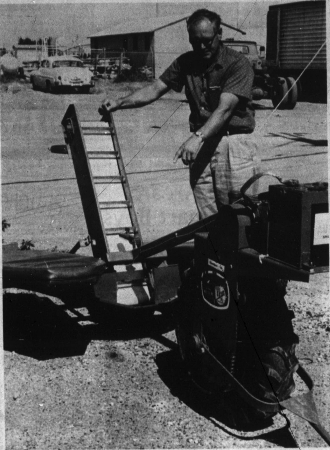
EXPLAINING THE OPERATION of a two-man cucumber picker tested by the Jorde Potato Co. on its 45-acre plot is Bud Jorde. The picker proved satisfactory for small five acre plots. The firm is planning to mechanize harvesting operations of the crop and intends to construct another type harvester using a conveyor belt. It was pointed out that the planned mechanization would reduce labor costs in harvesting the crop by approximately 35 per cent. (Staff Photo)
